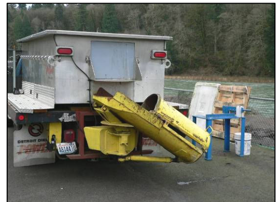
Photo 39: Nutrient Enhancement - salmon carcasses are also distributed by truck and chute system.
