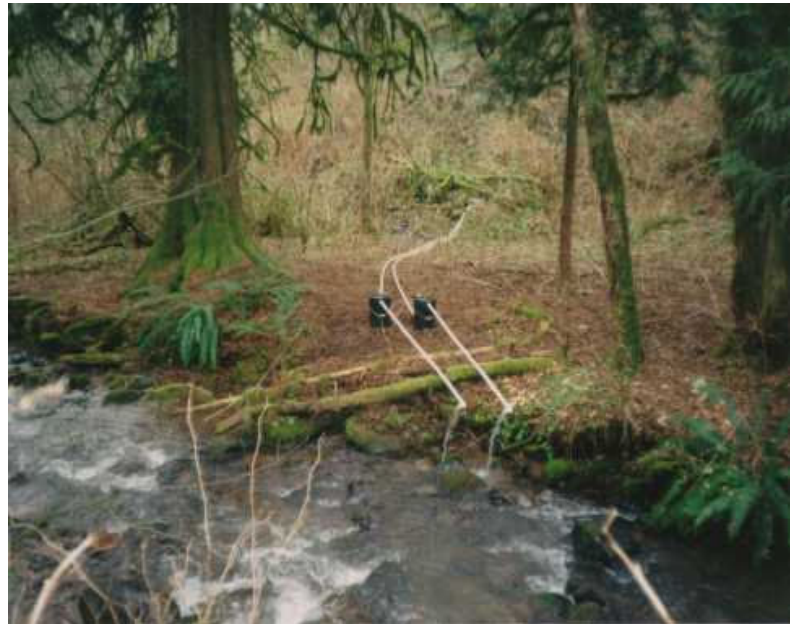
Photo 43: Egg Boxes - Remote Site Incubators (RSIs) installed on a tributary stream with spring water feed.
