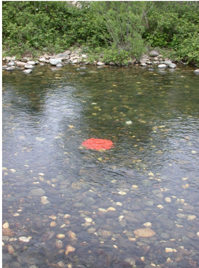
(red painted tracers for sediment transport study in the lower Yuba River)
