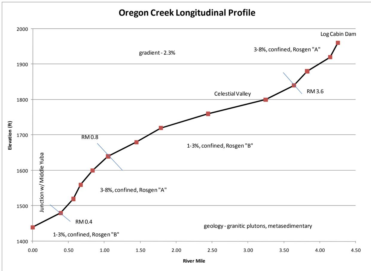
Figure 7.1.8-2. Longitudinal profile and channel classification of Oregon Creek.
