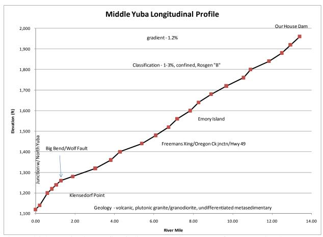
Figure 7.1.8-1. Longitudinal profile of Middle Yuba River between Our House Diversion Dam and the North Yuba River.
