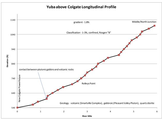
Figure 7.1.8-4. Longitudinal profile and initial channel classification of Yuba River between the New Colgate Powerhouse and the Middle/North Yuba junction.
