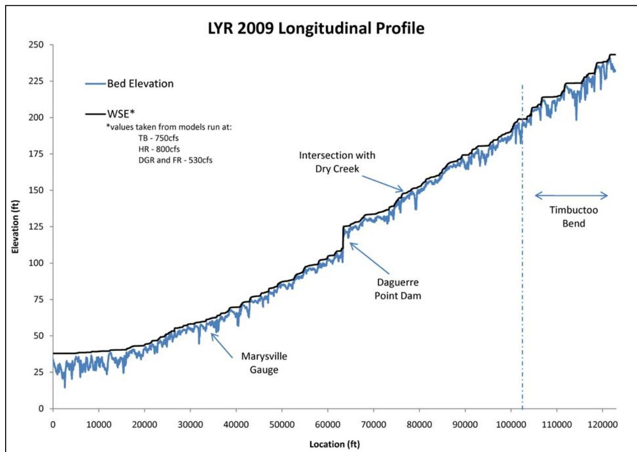
**Figure 7.1.8-5. Longitudinal profile of Yuba River below Timbuctoo Bend.**
