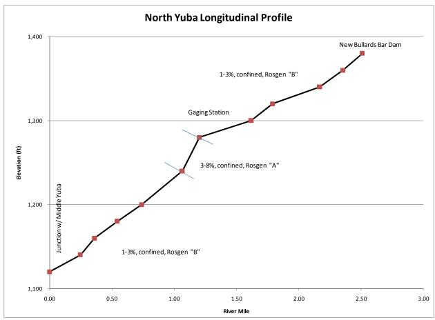
Figure 7.1.8-3. Longitudinal profile and initial channel classification of North Yuba between the junction with Middle Yuba and New Bullards Bar Dam.
