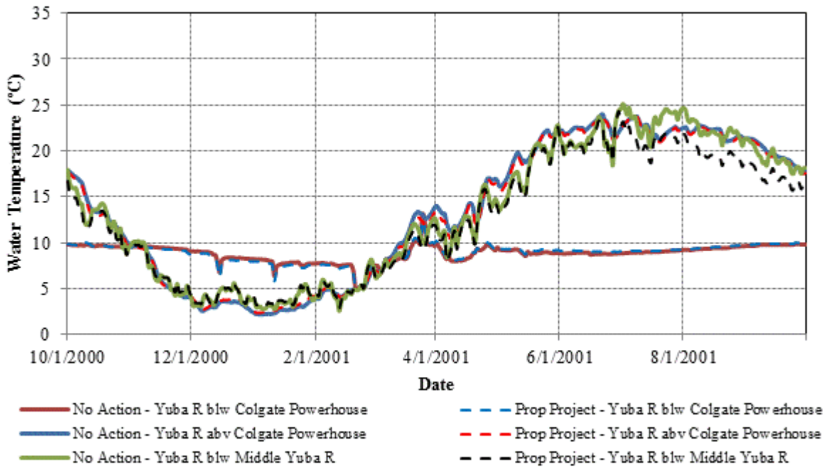
Figure 3.3.2-50. Simulated daily water temperatures for a representative dry WY (2001) at various locations along the Yuba River upstream of Englebright Reservoir.
