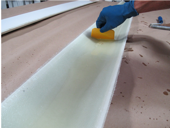
A) Initial creation of fiberglass antenna body.
