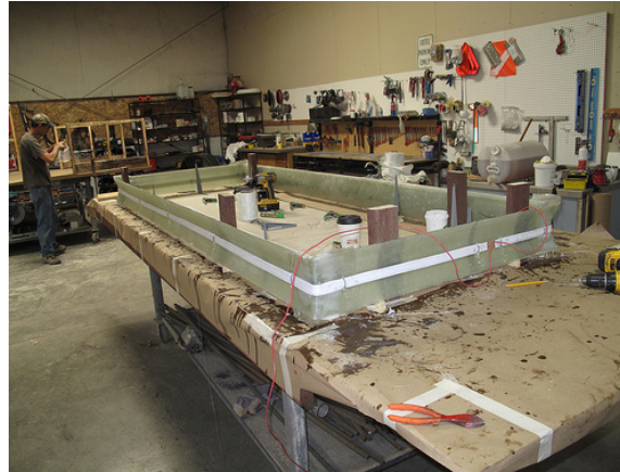
B) PIT antenna wire is embedded into the fiberglass layers.
