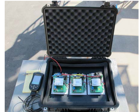
F) Series of 3 antenna logic 'detector' boards (in case) and single data logger on left. This is protected in a YCWA locked storage case onsite.
