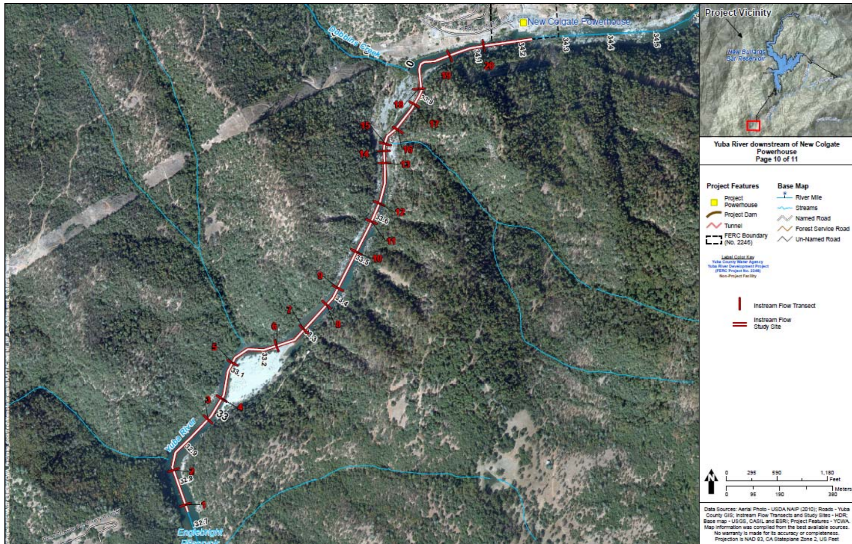
Figure 3.0-1. PHABSIM transects in the New Colgate Powerhouse Reach.
