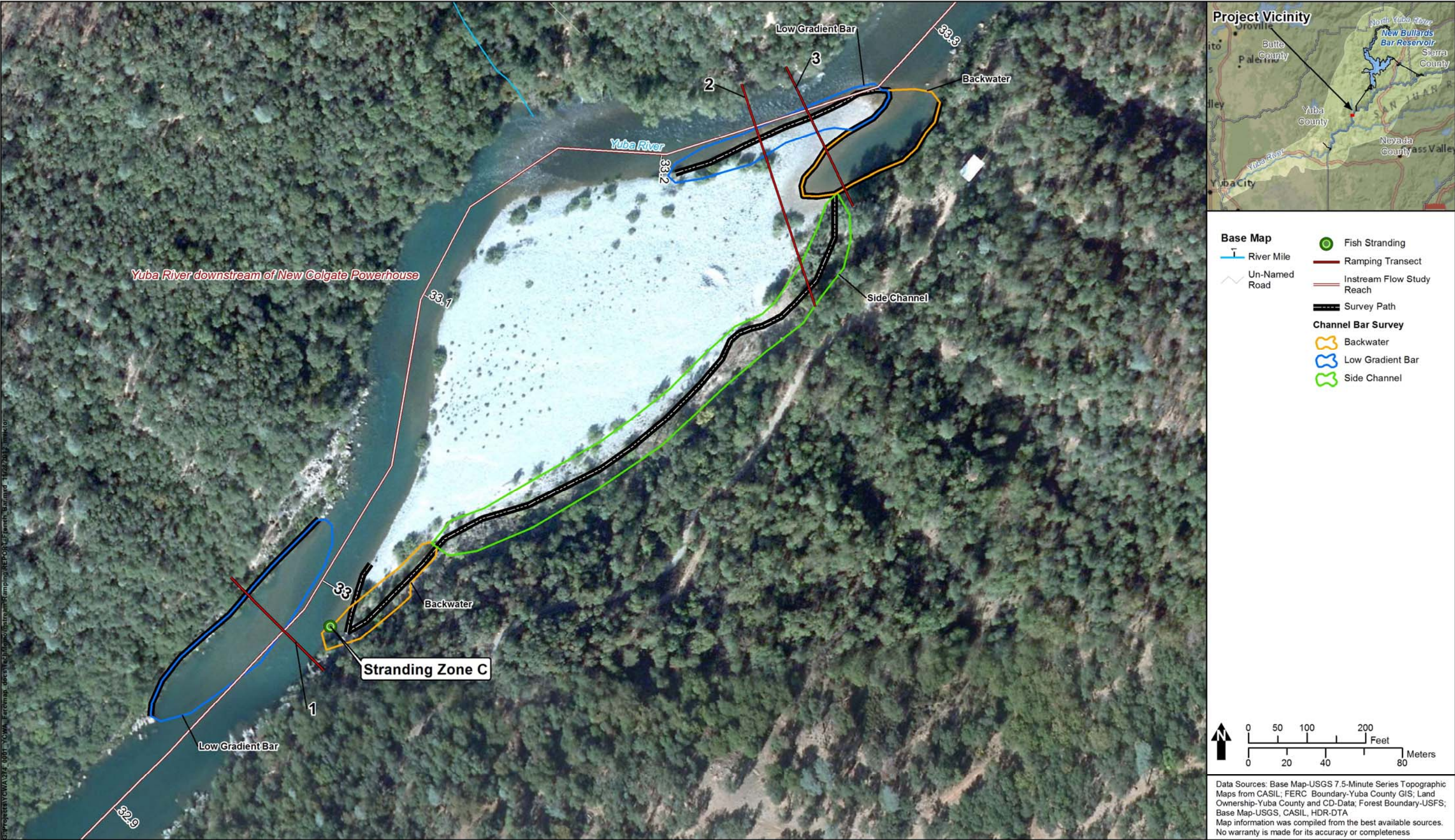
Figure 2.2-2. Location of French Bar downstream of New Colgate Powerhouse Reach. Hydraulic transects, bar habitat mapping, fish stranding survey routes and fish stranding observations are shown.
