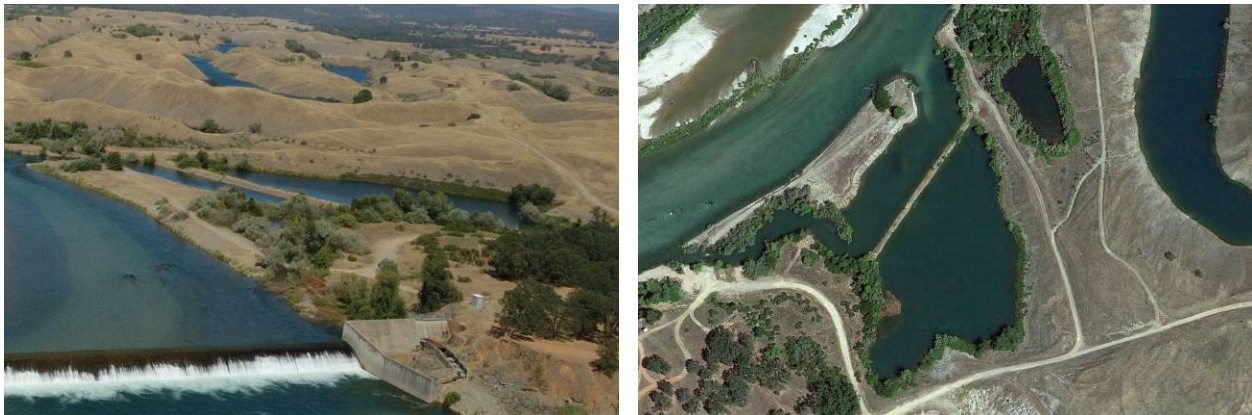
Figure 3.2-7. The South Yuba-Brophy Diversion. The image on the left shows the general location of the diversion (center of picture) relative to Daguerre Point Dam. The image on the right shows an aerial view of the bypass channel, rock gabion, and diversion pool.
