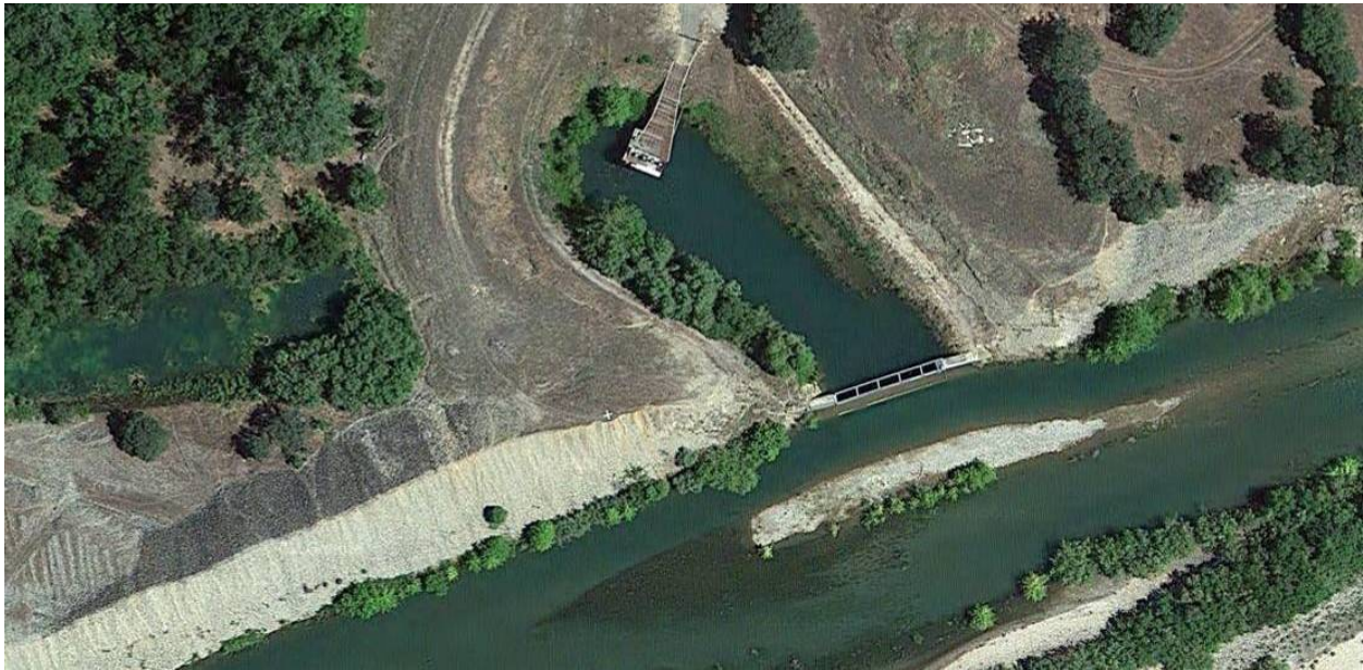
Figure 3.2-8. Browns Valley Diversion. Image shows the screen and diversion forebay.
